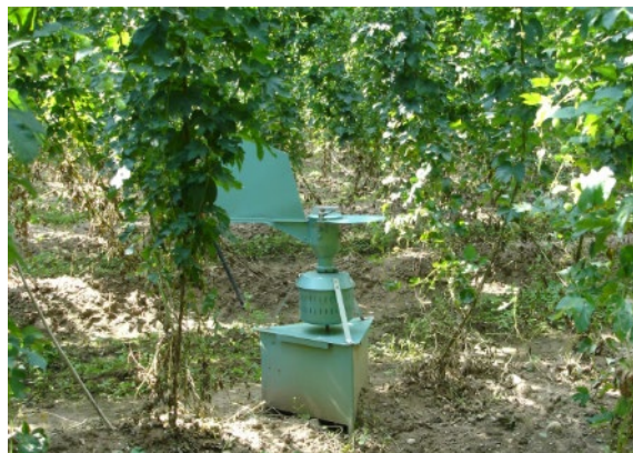
Figure 12.- Burkard spore trap for monitor downy mildew infection potential in hop gardens (Courtesy S. Radišek)
